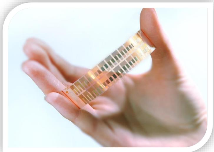
NanoFlex™ also supply the **CAVIARE™ Nanoband Array** electrode, a research-grade electrode which can be used to trial this exciting technology.
